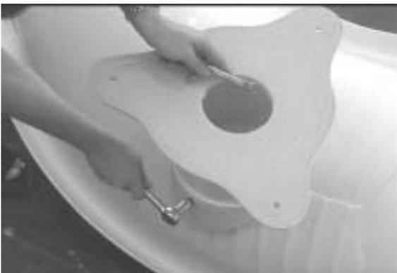
3. Secure on the inside of the pipe with 1/4" nut and corresponding washer using a 7/16" wrench. Repeat for all three holes.
