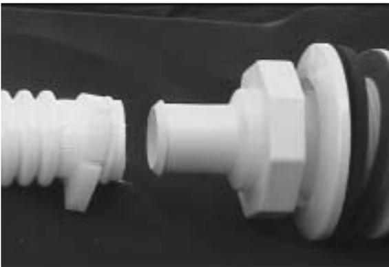
4. Slide the hose over the lipped flange of the adaptor fitting until the lip locks into the hose corrugation. Attach the plastic clamp, but do not secure too tight. You should be able to swivel the fitting inside the hose (in order to hand thread or remove the Zoomerang™ hose/adaptor fitting combination without tools).
