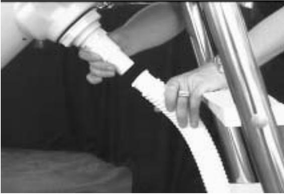
1. Wet one end of the hose and slide it onto the cone shaped fitting on the underside of the flume (Fully enclose the smaller cone). Secure with a plastic clamp by pinching together the interlocking teeth.
