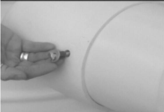
1. Align pre-drilled holes in the flume support pipe with those of the receptor on the underside of the flume.
